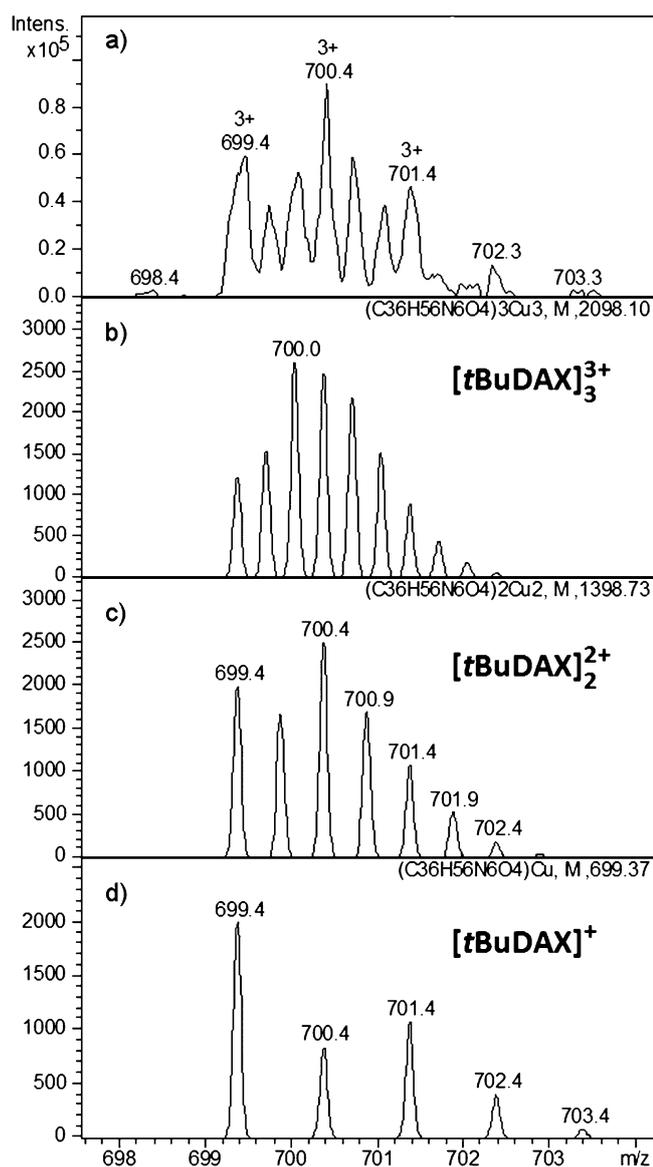
**Figure 3.** Enlargement of the signal at  $m/z = 700.4$  (top) and theoretical simulated pattern for several  $[\text{tBuDAX-Cu}]_n^{n+}$  species (below).
